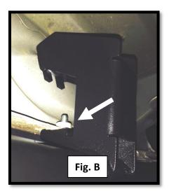
**Step 5:** After final positioning, start at the rear of the vehicle and tighten the lower portion of the bracket to 15-20 ft/lbs of torque. Continue this until all of the lower have been tighten then move to the top bolt and repeat the process.
