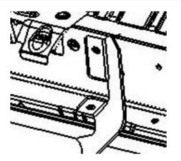
**<u>Step 4</u>** After final adjustment tighten all the lower mount first then the upper mounts. **<u>Step 5</u>**: Repeat steps 2-4 for the passenger side.
