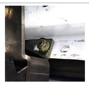
**Step 7:** After final adjustment, begin tightening the lower attachment points starting with the rear bracket working your way up to the front bracket. ( **20ft/lbs** )
