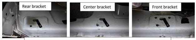
U-clip positioning. NOTE: Clips will also face forward for passenger side.
