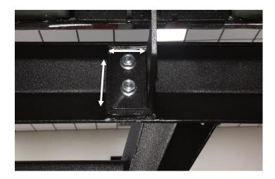
**Step 7:** Starting with the rear bracket, carefully push up from the bottom and position the rail snug under the body of the vehicle and tighten only one of the carriage bolts.
