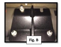
**Step 5:** Staring with the rear bracket, push up towards the pinch weld so the 3" main bar is as high and tight to the body as possible. Tighten all three 8mm flanged nuts.
