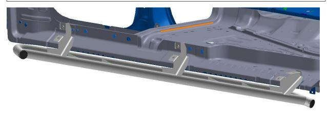
Step 5: Next, tighten the three lower bolts first, following with the three upper bolts.Step 6: Repeat steps 2-5 with passenger side.Step7: Your install is now complete.
