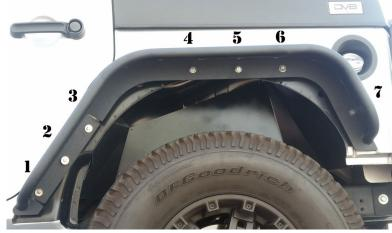
4) side you may need to use some force to manipulate the fender to align all the holes. Once all bolts in you can tighten them down. Note: Due to some variations in hole locations on the vehicles you may need to slightly enlarge holes with a drill. Use caution when drilling.
