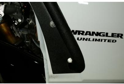
4b)bolts to go in. You will need the ratchet with the 13mm socket and combination wrench in 13mm during this process. Once all the screws are in place go ahead and tighten it down. Note: Due to some variations in hole locations on the vehicles you may need to slightly enlarge holes with a drill. Use caution when drilling.
