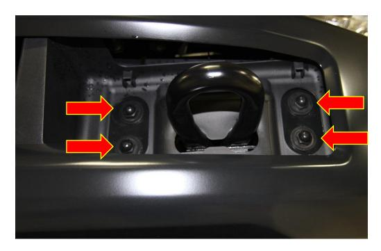
2. Next, with the help of someone holding the bumper in place, remove the four 15mm bolts from the bumper supports on both sides of vehicle.
