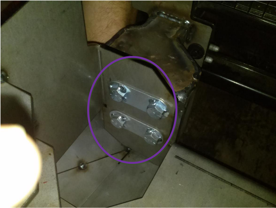
Figure 13b (bracket mounted to frame)
