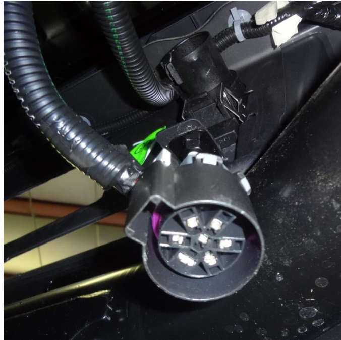
Figure 3a (ELECTRICAL HARNESS DISCONNECTED)
