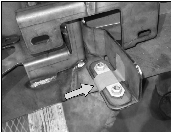
Figure 8 – OEM NUT PLATE PRE-INSTALLATION
