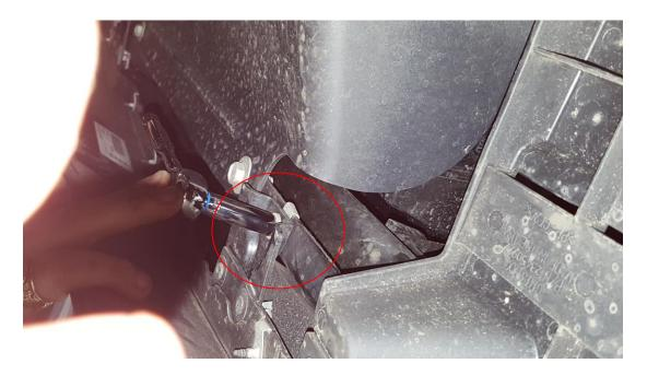
D. Using a 10mm socket and extensions, go through the grill and remove the two bolts holding it to the vehicle.
