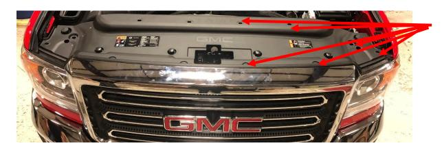
B. Once the cover is gone you will have access to remove the 4x 10mm bolts holding the top of the grill.
