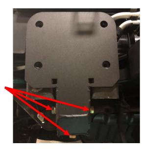
B. Use the OEM mounting bolts to attach the wench plate to the brackets.
