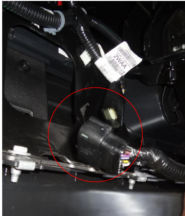
Figure 3(electrical harness disconnected)
