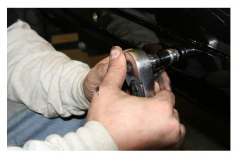
M. Tighten the bolt into the nutsert until it becomes snug in the rocker panel. DO NOT OVERTIGHTEN CAUSING THE INSERT TO SPIN!
