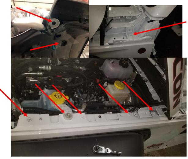
**5.** Remove the fender. While removing disconnect the running light/ turn signal harness behind the fender.
