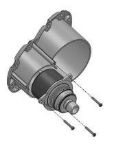
I. Install the light inserts with turn indicators into the cutout in the bumper. Use the <sup>3</sup>/<sub>4</sub>" length <sup>1</sup>/<sub>4</sub>" stainless steel button head, <sup>1</sup>/<sub>4</sub>" washers and hex nuts to fasten the insert through the holes shown below:
