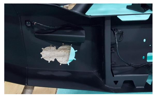
D. After ensuring sensors work in the current orientation, epoxy should be applied to the housing on the inside of the bumper and allowed to dry.
