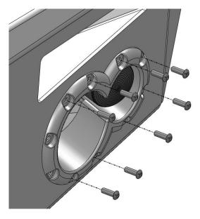
J. Install the Fab Fours fog lights onto the mounting brackets as shown below using the #8 button head screws, washers, and hex nuts.
