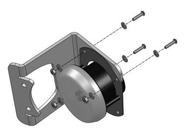
K. Install the fog light and bracket into the bumper using the remaining two holes available in the light insert. Use the 1-1/2" length ¼" stainless steel button heads with ¼" washers and nuts.
