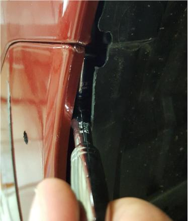
14. Remove lower fender lining screw and peel back lining to expose 10mm bolt. Remove this bolt.
