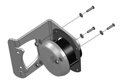
K. Install the fog light and bracket into the bumper using the remaining two holes available in the light insert.
