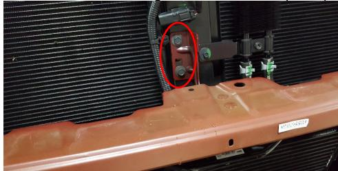
19. Reattach grill to truck. The pins must be installed into the grill before pressing into the truck.
