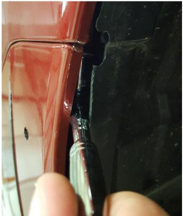
15. Carefully pull form outside of fender to release clips and remove valance.
