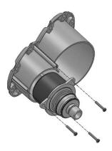
I. Install the light inserts with turn indicators into the cutout in the bumper. Use the ¾" length ¼" stainless steel button head, ¼" washers and hex nuts to fasten the insert through the holes shown below:
