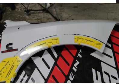
Cut Template 9 (DS\_FEN\_4) is placed beside DS FEN 3 and continues the previous cut template. Start by placing the circular locating hole on the third-from-front inner fender mount hole as shown. Again, take care to match the template contour to the contours around the mount hole, then roll the template upwards. Take care to match the blue, hashed contour line with the overall fender curvature. Continue to lay the template up, smoothing out any bubbles or wrinkles that may form.
