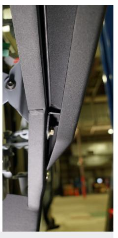
Install seal on mounting edge of all flares. See Appendix A for install instructions if necessary. Insert bolts through slots in fender flare mounts and fasten into weld nuts on base fender. Bolt install points are indicated by red circles.
