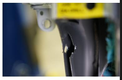
Drill ½" holes on remaining template pieces on rocker channel stepping up from a 1/8" bit to full size. For the hole on the outer surface of the truck, cut back the region around the hole on the NEXT LAYER inboard with respect to the truck (indicated on photo). Cut and grind any of these inner layers as much as needed to get the parts to slide into position correctly.
