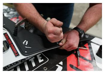
Use an appropriately sized centerpunch to mark each hole (7 holes total). Remove base fender from OEM fender and set aside. Starting with a 1/8" drill bit, step up to 3/8" diameter holes. Apply rust trap to every cut/drilled edge and allow to dry.
