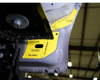
Cut Template 2 (DS\_CAB\_2) is applied to the front of the rocker channel as shown. Place the large oval cutout over the large oval hole on the rocker surface, starting on one side and smoothing around the hole. Roll the template upwards using the outboard edge of the surface as a guide for the template edge.
