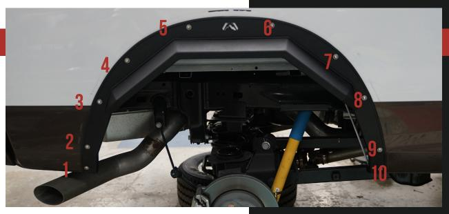
Remove fender completely from side of truck and set aside. Stepping up from a 1/8" bit, drill 3/8" diameter holes at every location marked with the centerpunch (10 holes total). Apply rust trap to every cut/drilled edge at this point and allow to dry.
