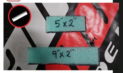
Remove the rocker plates and set aside. From the blue, foam packing material that came with this product, cut sections out like the ones in the photo to the left. Insert these foam pieces into the rocker channel as shown. These pieces will block the foam from pushing back into the rocker channel and direct the foam upward into the upper part of the channel.
