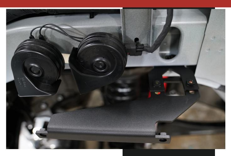
Place the bracketry template DS/PS\_BRKT\_1 on the frame of the truck as shown. Drill through indicated hole location, stepping up from a 1/8" bit to 3/8" diameter. Apply rust trap to every cut/drilled edge and allow to dry. Lay small nut plate inside of the tubing as shown and use the hardware specified to fasten it to frame.
