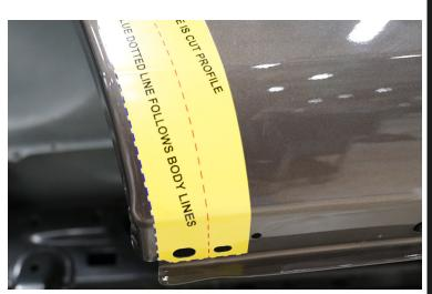
Cut Template 11 (DS\_FEN\_6) is placed on the rear fender, behind the rear axle. Starting from the bottom, place the two oval-shaped locating holes on the two oval-shaped holes. After smoothing out bottom area of template, roll the upper template portion upwards taking care to keep the blue, hashed contour line in line with the fender curvature. When you get to the top of the template, roll the tab inboard and place secondary locating hole on the closest inner fender mount hole.
