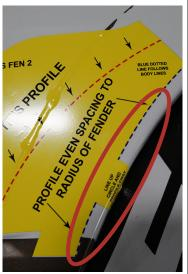
Cut Template 6 (DS\_FEN\_1) is placed on the valence piece from directly below the headlight. Starting on the end of the part (where the locating pegs protrude from), match template edges to cutout edges on face of part, then roll the template around to the front face. Roll the remaining tab around the bottom edge to complete placement.
