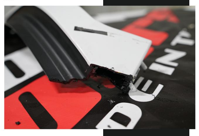
Using a body saw (or other appropriate tool), cut through the part at the template DS\_FEN\_1 cut line beginning on the narrower side. The cut should look as if a plane separated the two pieces.
