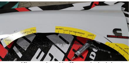
\*Clean up edges with a [flapper wheel, grinder, etc...
