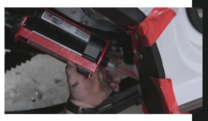
Re-install the rocker channel plates. Cover all exposed gaps or edges with duct tape to seal the foam inside the channel. Using the hole shown, insert the foam into the rocker channel cavity. Wait for the foam to expand. Remove tape, then grind/sand any protruding edges very carefully.
