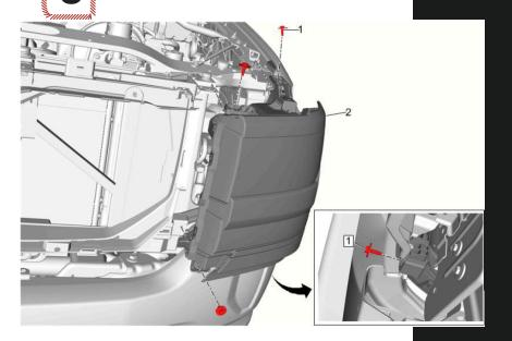
Locate and remove the (4) fasteners that attach the headlights to the core support and fender.
