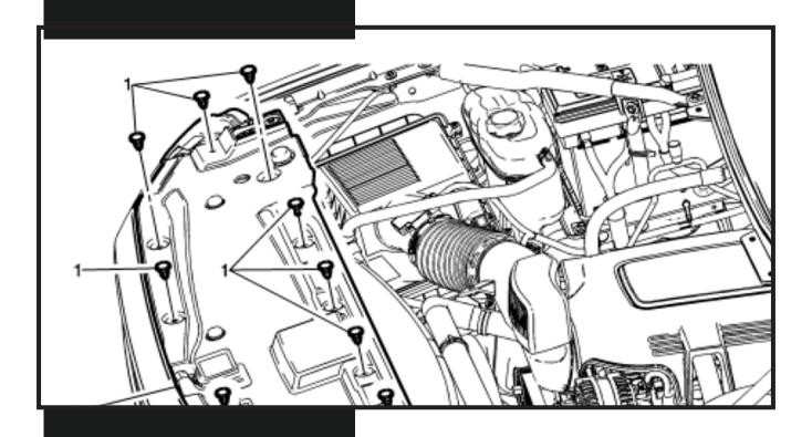
Locate and remove the (11) push pins using a body panel tool. Bag and tag the pins and cowl.
