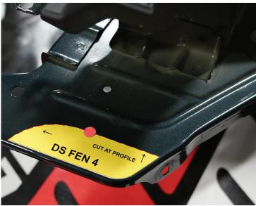
Cut Template DS FEN 4 is applied to the front side of the driver's side front fender ahead of the fender well opening. Align the edge of the template with the fender profile and the locating hole as shown.
