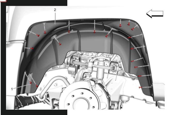
Using a T15 Torx bit locate and remove the fasteners attaching the OEM inner fender coverings to the fender. Bag and tag hardware, it will be reused. Repeat process on other side of the vehicle.
