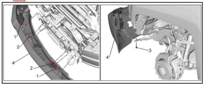
Looking down from the top of the bumper, locate and remove the (6) fasteners that attach the bumper to the frame horns. From under the bumper locate and remove the (3) fasteners per side that attach the bumper support brackets to the bumper and frame.
