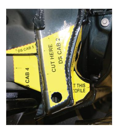
Cut Template DS CAB 2 is applied to the front of the rocker channel as shown. Place the circular cutout over the hole on the rocker surface. Roll the template upwards using the outboard edge of the surface as a guide for the template edge. DO NOT conform the template to the step in the sheet metal, this is NOT necessary.
