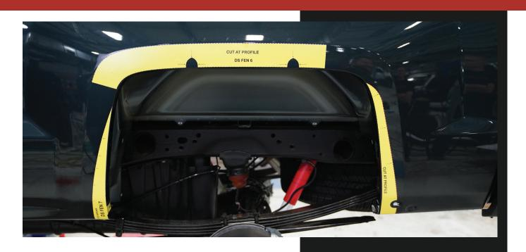
Cut Template DS FEN 7 is applied to the lower front of the driver's side rear wheel well opening. Starting at the bottom, work your way up the fender with the template aligning the location hole with the nut insert and then the inside edge of the wheel opening.
