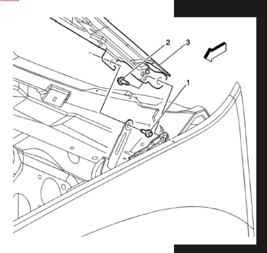
Locate and remove the (2) bolts that attach the hood brackets to the hinge. Bag and tag bolts. Place hood in a safe padded location.
