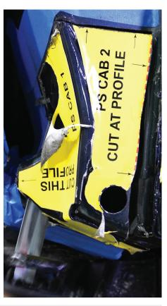
Begin the cutting process with DS CAB 1. Starting from the bottom, working up use a cut-off wheel and follow the red dashed lines on the template and cut through the (2) sides of DS CAB 1. Next, using a large reciprocating saw, cut vertically through the inner structure of the rocker channel. Be careful not to cut above the template line.
