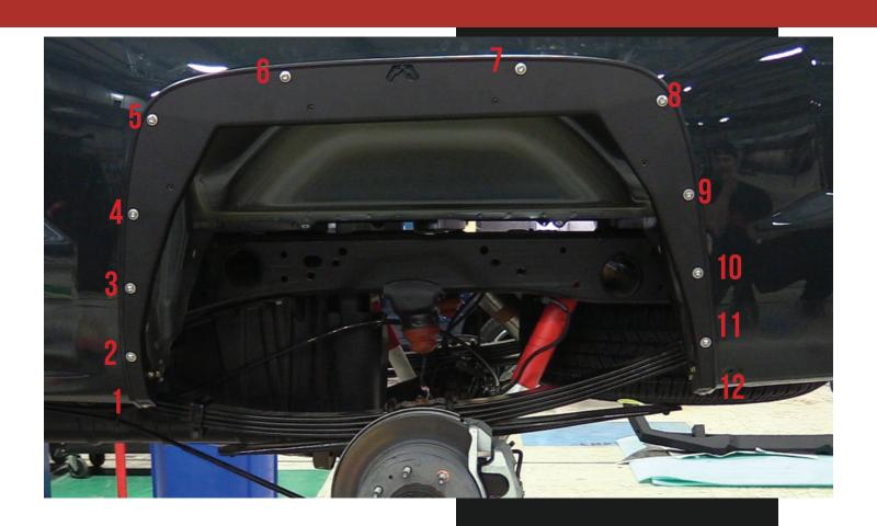
Place fender back on the truck. At this time loosely bolt locations 5,6,7, and 8 using the provided 5/16" hardware. Continue with installing the rest of the hardware in locations 1-4 and 9-12 using the 5/16" hardware provided.
