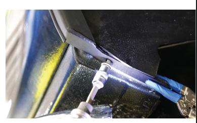
Apply seal to front base fenders as shown in Appendix. To install the front fender bases, have someone hold the base against the front OEM fender aligning the outer profile of the Fab Fours base with the profile on the OEM fender. Mark the center top two holes. Remove the base and drill out the two marked holes in the OEM fender starting with a smaller drill bit and working up to the included 17/32" drill bit.
