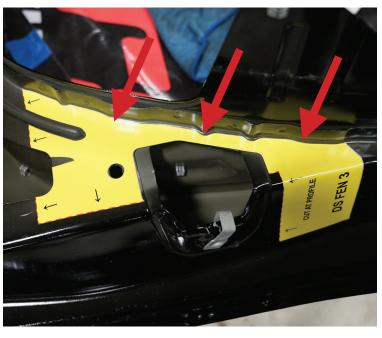
Cut Template DS FEN 3 is placed on the backside of the driver's side front fender. Start applying the template by lining up the profile shown with the red arrows. Then work the template across matching the locating hole with the one on the fender.
