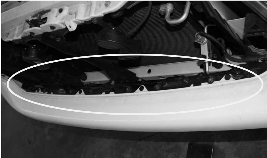
Figure 5 - Center Fascia Fasteners
