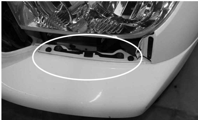
Figure 6 - Outer Fascia Fasteners
