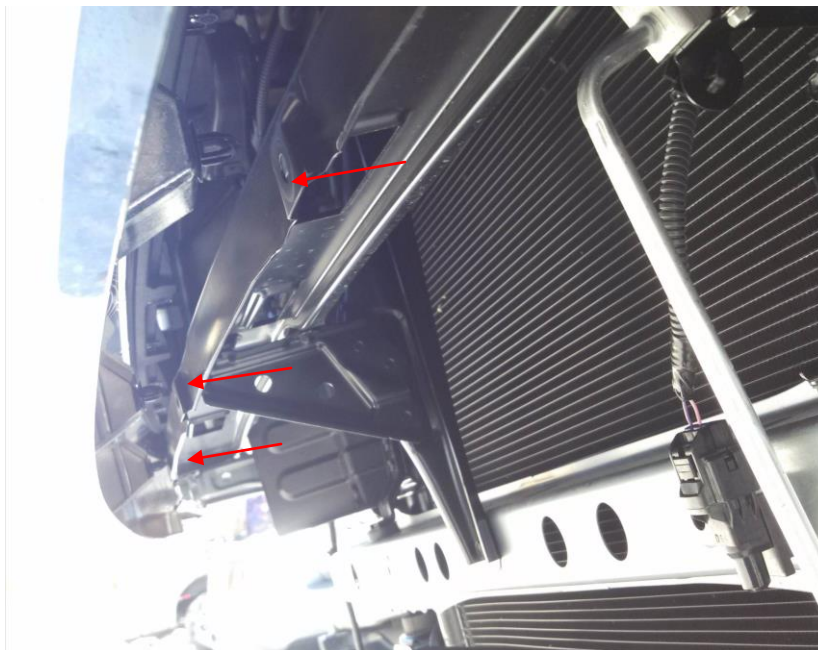
Figure 6 - Grill Plastic Clip Locations
