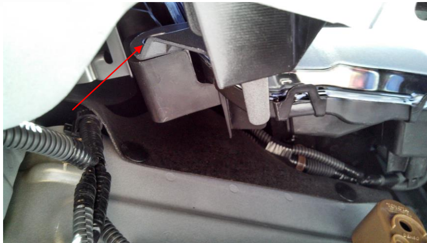
Figure 5 - Pop Clip Location Headlight to Plastic Fascia
