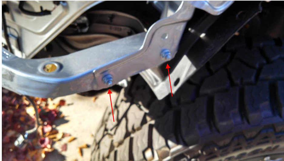
Figure 9 - Fascia Brace Nuts
