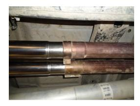
6) Place the inlet pipes of the new FlowFX muffler **#7430404-461** into the factory front pipes and connect the hangers on the muffler to the rubber mounts on the vehicle. Be sure the muffler is fully forward and seated. Tighten the clamps enough to hold.
