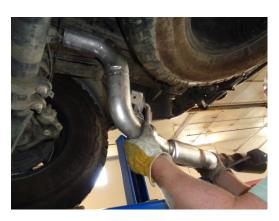
8) Re-install the tailpipes into the muffler outlets. Be sure that they are fully seated and tighten the clamps enough to hold but still allow for adjustment.
