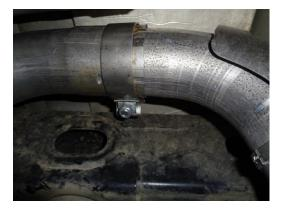
2) Loosen the two clamps connecting the tailpipes to the muffler at the over-axle slip-fit connections. Carefully slide the tailpipes toward the rear to remove from the muffler. Allow the pipes to hang until installation of the Flowmaster muffler.
