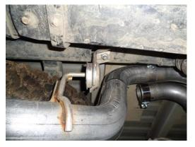
3) It may be necessary to unbolt the forward hanger on each tailpipe from the frame to allow the tailpipes to slide out of the muffler outlets.
