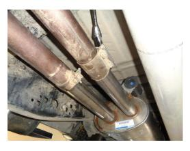
4) Support the muffler with a stand and loosen the clamp on each of the two front inlet pipes using a 15mm socket wrench. Then slide the muffler toward the rear of the vehicle to disconnect the inlet pipes and the hangers from the rubber mounts on the vehicle. Lower and set the muffler aside.
