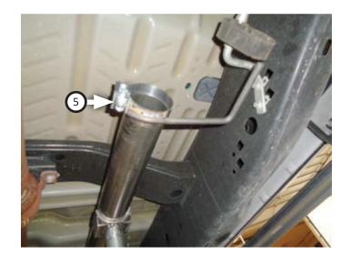
8. If your front frame mount doesn't align to properly connect to frame hanger, remove (x2) screws attaching mount to frame, move (x2) plate nuts to forward set of holes and remount hanger to frame.
