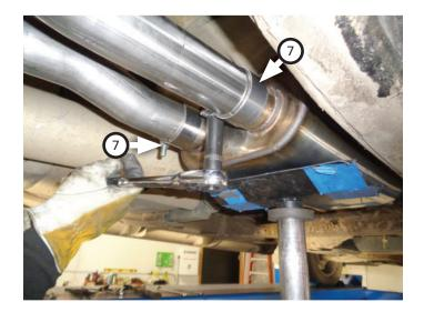
13. Adjust exit pipes to desired distance from body, so angle cut on tips are properly positioned. Rotate bracket so it lays flat against inside of vehicle frame then use a center punch to mark center of (x2) holes on frame. Move hanger aside and drill each mark using a ¼" drill bit. Finally use (x2) **bolts (9)** to secure hanger to frame and tighten securely.
