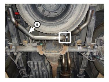
16. Place (x2 ea.) clamps (12) onto side exit pipes (7) then connect them to rear tailpipes. Tighten clamps just enough to allow for adjustment.
