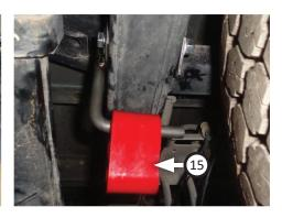
13. Route **right tailpipe (4)** over rear axle then connect it to passenger side muffler outlet. Insert wire hanger into stock mount to complete connection. Tighten clamp just enough to allow for adjustment.
