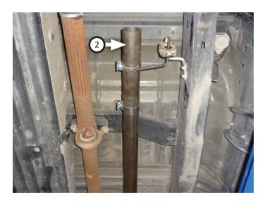
11. Place **clamp (13)** onto **muffler (3)** inlet then connect it to inlet/extension pipe. Place (x2) **clamps (12)** onto muffler outlets. Tighten front clamp just enough to allow for adjustment.
