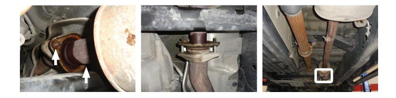
4. Disconnect factory muffler wire hangers (x2) from isolators on vehicle frame.
