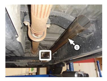
Place clamp (13) and front clamp hanger (9) onto extension pipe (2). Hang assembly onto vehicle frame and connect to inlet pipe.
