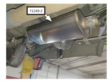
9. Route **tailpipe assembly (26754M)** over axle and connect it to muffler outlet. Mount wire hangers into isolators (x2) then tighten clamp enough to allow for adjustment.
