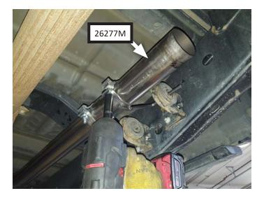
Place clamps (x2) (MC300BS) onto each end of FFX muffler (71249-Z) then connect it to extension or inlet pipe. Tighten front clamp enough to allow for adjustment.
