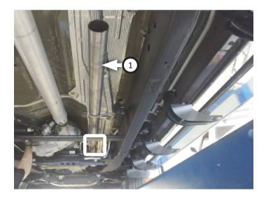
9. If applicable, place **clamp (12)** onto **extension (2)** then connect it to inlet pipe. Tighten clamp just enough to allow for adjustment.
