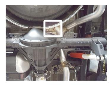
4. Remove bolt and mount securing driver side tailpipe then remove it from vehicle. Retain bolt and mount for later use.
