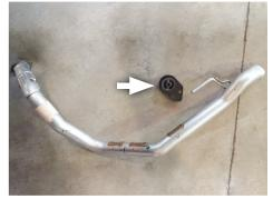
5. Cut tailpipes just behind factory muffler.
