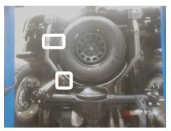
16. Adjust exhaust components for fit; maintaining ½" clearance and compensating for suspension, travel and vibration then tighten all clamps. Finally, fit (x5) hanger keepers (10) onto each sideways hanger.
