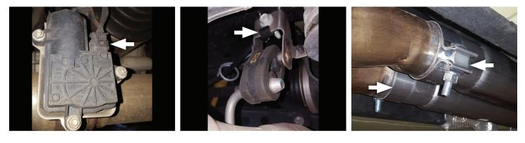
4. Carefully lower stands at vehicle rear and with help from an assistant, slide system back off the head pipes and lower system from vehicle.
