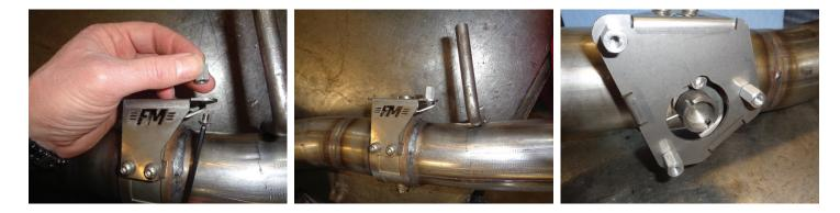
9. Insert (x3 ea.) **screws (10)** through actuator and **flat washers (11)**. Place actuator onto tailpipe valve mount then tighten screws to fasten assembly.
