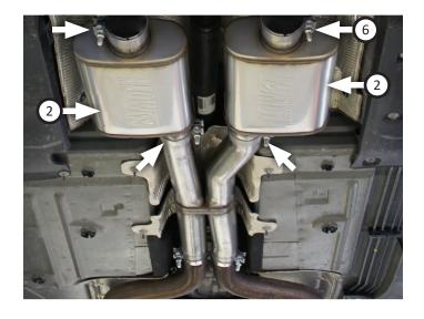
13. Transfer hangers from step 3 onto **right and left tailpipes (3, 4)**. Connect them to mufflers, insert wire
