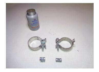
Place clamp (3) onto muffler (1) then connect it to factory outlet, lining inlet pipe notch with outlet tab. Insert wire hanger into isolator then tighten clamp enough to allow for adjustment without covering tab.
