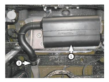
Place clamp (3) onto muffler outlet then connect tailpipe assembly (2) to it. Insert wire hanger into rubber hanger then tighten clamp just enough to allow for later adjustment.
