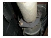
2) Support the muffler with a stand and unbolt the flanged connections behind the catalytic converters. (Save the nuts, bolts and metal gaskets for the installation.) It will be necessary to take a 12mm socket and unbolt the hanger bracket from the frame that holds the head pipe and muffler assembly up (save bracket and bolts, you will reinstall with new system). Remove muffler and set aside.
