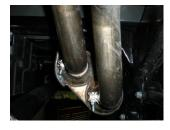
5) Place the provided 2½" clamps onto the muffler outlets and re-install the tailpipes into the muffler outlets. Be sure to line up the tabs on the tailpipes with the notches on the muffler outlets. Tighten the clamp securely.
