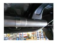
2) If installing the system on a Crew Cab truck with a 6.5' bed, place extension pipe **#36065S** onto the back of the **#36064S** inlet pipe, place a provided clamp onto the slip-fit and tighten enough to hold in position. This extension pipe will not be used on Double Cab or Crew Cab-5.5' bed models.
