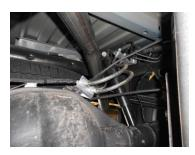
6) Place left front tailpipe section **#86094S** into position over the rear axle and slide into the left muffler outlet. Place a supplied 2-1/2" clamp onto the back of the pipe. Place left rear tailpipe section **#86404S** onto the front section, and connect the hanger welded to the rear of the pipe into the rubber hanger installed in step 3 above. Pipe should be centered between the shock and the spare tire when adjusted. Tighten the clamps just enough to hold in position.
