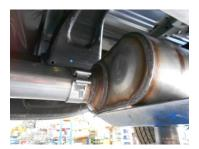
3) Place a supplied 3 ½" clamp over the inlet of the muffler and then slide the inlet of muffler onto the back of the inlet pipe. Use a stand to support the muffler. Tighten the clamp just enough to hold in position.
