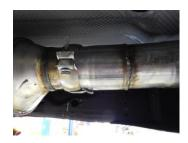
1) Place inlet pipe assembly **#36064S** into position onto the ball connection behind the catalytic converter. Reinstall the clamp onto the ball connection and tighten enough to hold, but still allow for a small amount of adjustment. Connect the hanger on the pipe to the rubber mount on the vehicle.
