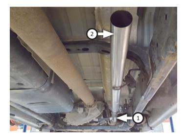
9. Place **clamps (x3) (10)** onto **muffler (3)** then connect it to rear inlet pipe. Adjust and level muffler then tighten all clamps on inlet assembly just enough to allow for final adjustment after install.
