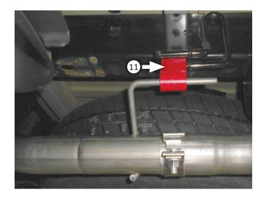
12. Place **clamp (10)** on **left rear tailpipe (6)** then connect it to left front tailpipe. Insert wire hanger into rubber hanger then tighten clamp just enough to allow for adjustment.
