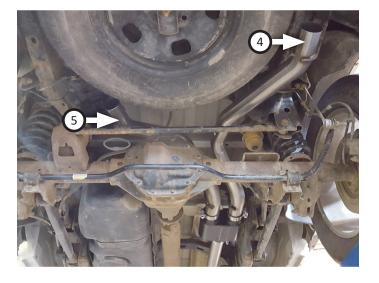
11. At rear of frame on driver side of vehicle (next to spare tire), is a pair of attached hanger mounts. Place **rubber** hanger (11) onto inner hanger.
