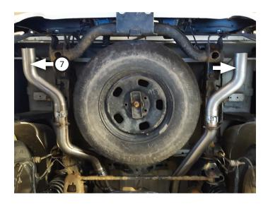
14. Place **stainless tips (9)** onto exit pipes and tighten inlets. Rotate exit pipes and tips to desired distance from body or bumper, so angle cut on tips are properly positioned.
