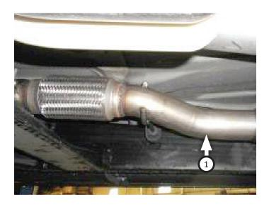
7. If applicable, place clamp (6) onto muffler (3) then connect it to inlet pipe. Tighten clamp just enough to hold parts.
