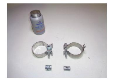
6. Place factory ball clamp (removed step 4) onto **inlet pipe (1)** then connect it to catalytic converter. Insert wire hanger into isolator and tighten clamp just enough to hold parts.
