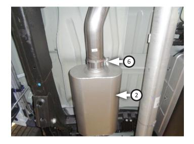
8. Place **clamp (6)** onto **over-axle pipe (3)**, route it over axle then connect it to muffler. Insert wire hangers into isolators then tighten clamp enough to hold parts.
