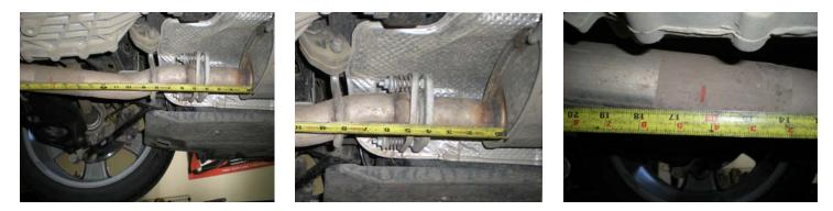
2) Begin by measuring back 16 ¼" from the edge of both factory mufflers and make a mark on the pipes (see photos above). Once you have double checked that the measurements are correct, cut both pipes through at the marks. Remove the two hangers on each tailpipe assembly from the rubber mounts on the vehicle and remove the tailpipe assemblies from the vehicle. Carefully deburr the end of the pipes with a file or die grinder.
