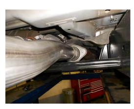
2) Place the inlet pipe onto the back of the existing OEM head pipe and fasten using the 3/8" x 2.00" bolts, nuts and washers provided in the hardware kit. Tighten just enough to hold in place, but still allow for adjustment.
