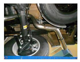
4) Install a provided clamp onto the muffler outlet. Then place tailpipe **#26575S** into position over the axle and into the muffler outlet while also connecting the hangers on the pipe to the rubber mounts on the vehicle. Tighten the band clamp enough to hold, but still allow for adjustment.
