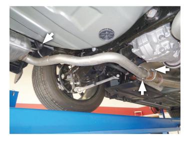
4. Support right side muffler and loosen clamps at slip fit connections behind catalytic converters. Unclip ground strap from middle hanger then slide system off of head pipes and set it aside.
