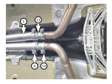
13. Place (x2) clamps (5) onto scavenger pipe (1) inlets then connect it to head pipes withoffset outlet pipe oriented to passenger side). Level and center assembly in drive line tunnel then tighten clamps enough to hold parts.
