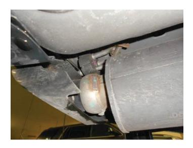
5. Remove (x3 ea.) nuts securing actuators to mounts on tailpipes. Remove actuator and spring from mount on each tailpipe.
