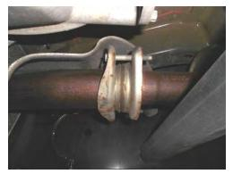
3) Support the muffler with a stand and remove the two bolts at the front flange connection. Now, with the help of an assistant, slide the exhaust system to the rear to disengage the hangers on the exhaust from the rubber mounts on the vehicle. Once free, the assembly can be removed by working it forward over the rear axle (If you are working on the ground it may be easier to cut the tailpipe off at the rear of the muffler to simplify removal).
