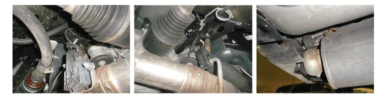
4. Remove (x3) nuts securing actuator to mounts then remove actuator and spring from mount on each tailpipe.
