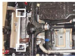
4. Loosen clamp at muffler inlet connection above rear axle then remove muffler from vehicle.
