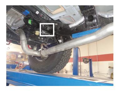
7. Loosen clamp at resonator inlet and remove resonator assembly from vehicle. Retain clamp for later re-use.
