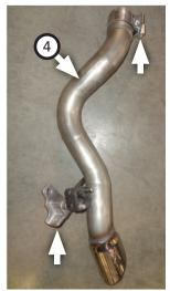
6. Remove stock resonator assembly from rubber isolator with a pry bar and retain for later re-use.
