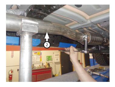
Place clamp (5) onto over-axle pipe (3), route it over and into inlet pipe. Insert wire hanger into isolator on vehicle then tighten clamp just enough to allow for adjustment.
