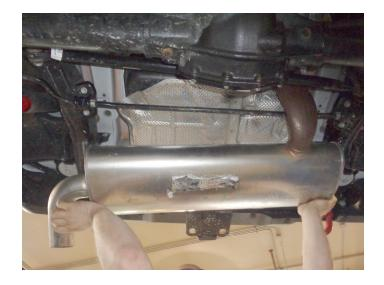
5. Transfer driver side mount and clamp from factory muffler to **tailpipe (4)**.
