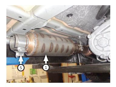
9. Place **inlet pipe (2)** into muffler, making sure bend is oriented upwards for maximum clearance. Tighten clamp just enough to allow for adjustment.
