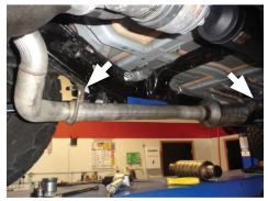
7. Remove resonator assembly from vehicle and retain clamp for re-use.
