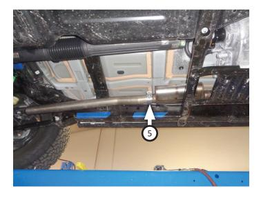
12. Place clamp (5) onto over-axle pipe (3) then connect it to front pipe while pushing wire hanger into rubber isolator on vehicle. Tighten clamp just enough to allow for adjustment.
