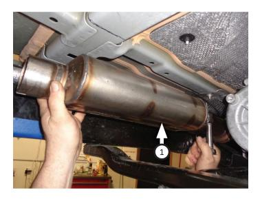
11. Place **clamp (5)** onto resonator then connect front pipe to it. Make sure front pipe bend is oriented upwards, then tighten clamp just enough to allow for adjustment.
