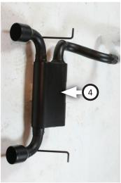
6. Remove wire hanger on resonator assembly from isolator, and loosen bolt on clamp at resonator inlet.
