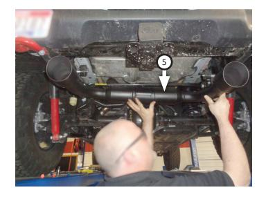
14. Place factory (driver and passenger side) hanger mounts into position, then reinstall and tighten factory bolts.
