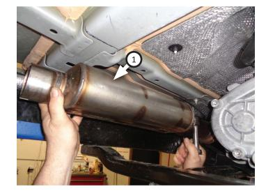
11. Place **clamp (6)** onto front inlet pipe then connect it to resonator. Make sure front inlet pipe bend is oriented upwards for maximum clearance. Tighten clamp just enough to allow for adjustment.
