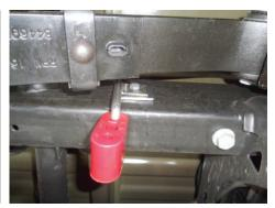
11. Route **left front (4)** and **right tailpipes (6)** over axle then connect them to muffler. Insert wire hangers into isolators then tighten clamps just enough to hold parts.
