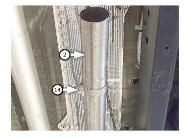
9. Place clamp (14) onto muffler (3) then connect it to inlet or extension pipe. Tighten clamp just enough to allow for adjustment then place (x2) clamps (13) onto muffler outlets.
