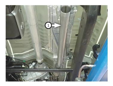
9. For applicable models, place **clamp (13)** onto **extension pipe (2)** then connect it to inlet pipe. Tighten clamp just enough to allow for later adjustment.
