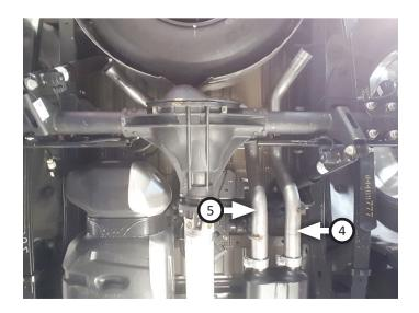
16. Place clamp (9) and isolator (removed step 6) onto left rear tailpipe (7) then connect it to left front tailpipe. Fasten isolator with bolt then tighten clamp enough to allow for adjustment.
