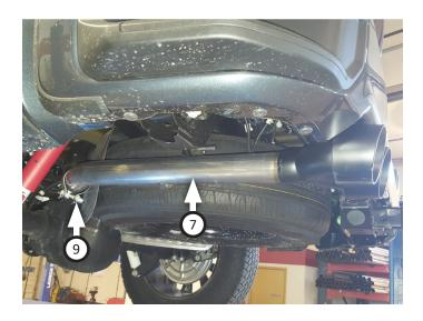
17. Place clamp (9) and isolator (removed step 8) onto right rear tailpipe (6) then connect it to right front tailpipe. Fasten isolator with bolt then tighten clamp enough to allow for adjustment.
