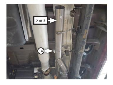
9. Place clamp (14) onto muffler (4) inlet then connect it to extension pipe. Tighten clamp just enough to allow for adjustment then place clamps (x2) (15) onto muffler outlets.
