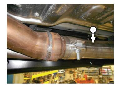
Place clamp (14) onto extension pipe (2 or 3) then connect it to inlet pipe. Connect wire hangers to isolators then tighten clamp just enough to allow for adjustment.
