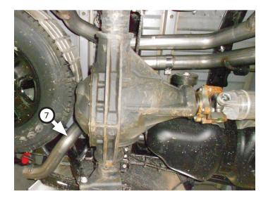
**NOTE:** This kit includes both side and rear exit pipes. A side exit is preferable for towing purposes, to avoid blowing fumes in or on vehicles you may be towing (eg: RV trailer, boat, etc). Otherwise, complete step 13 using **rear exit pipes (9)** in place of side exit pipes.
